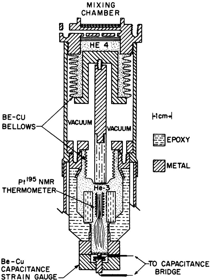
Figure 1: Schematic diagram of the Pomeranchuk cell used in the discovery of superfluidity in  $^3\text{He}$ . Superfluid  $^4\text{He}$  is added to the upper bellows assembly under pressure, forcing the lower bellows into the  $^3\text{He}$ -filled region. The capacitive pressure transducer is at the bottom. (Reproduced with permission from reference 11).
