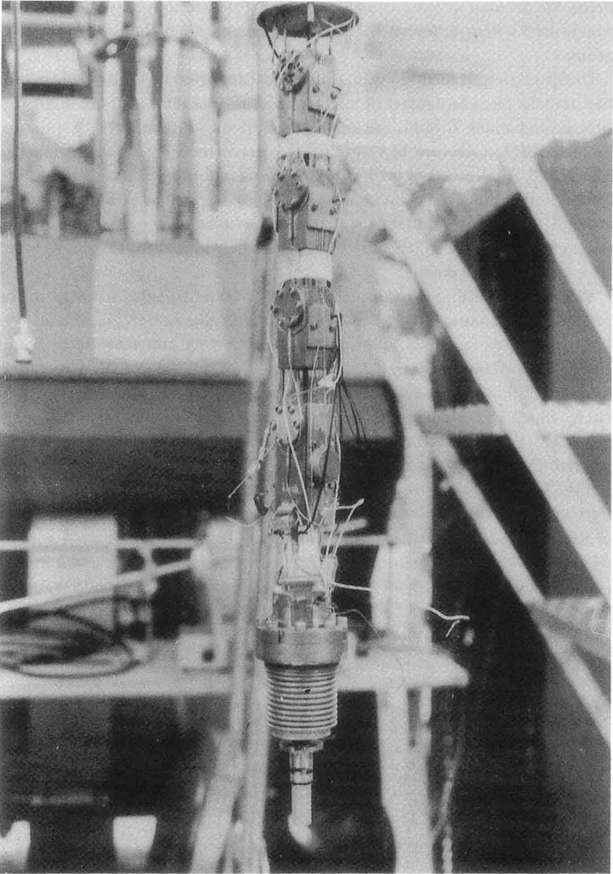
Figure 2: Photograph of the lower portion of the dilution refrigerator used in the discovery, showing the heat exchange column and, at the bottom, the mixing chamber with the  $^4\text{He}$  bellows chamber and piston for the Pomeranchuk cell attached.
