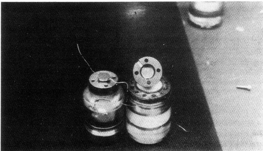
Figure 3: Photograph of the capacitive pressure transducer for the  $^3\text{He}$  cell during assembly. The moving capacitor plate attached to the metal diaphragm is seen at the left, while the stationary plate is on the right.
